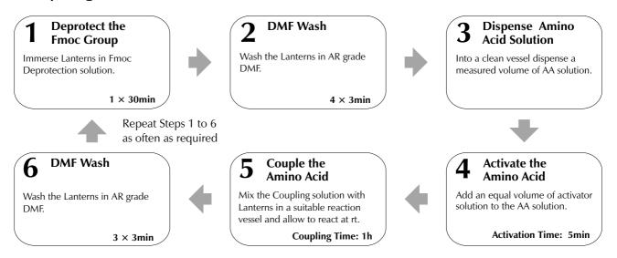
SynPhase D-series Lanterns require typical working volumes of 500µL. Actual volumes depend upon the dimensions of the reaction vessel and the number of Lanterns used. The procedure may require slight optimization
